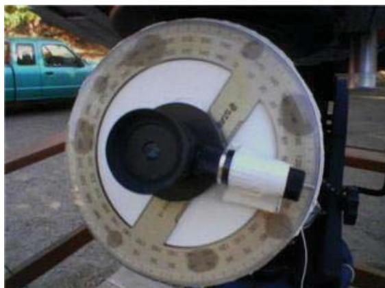
Figure 2. A protractor-pointer designed by Johnson to measure the position angle of the double star STF 2079.
