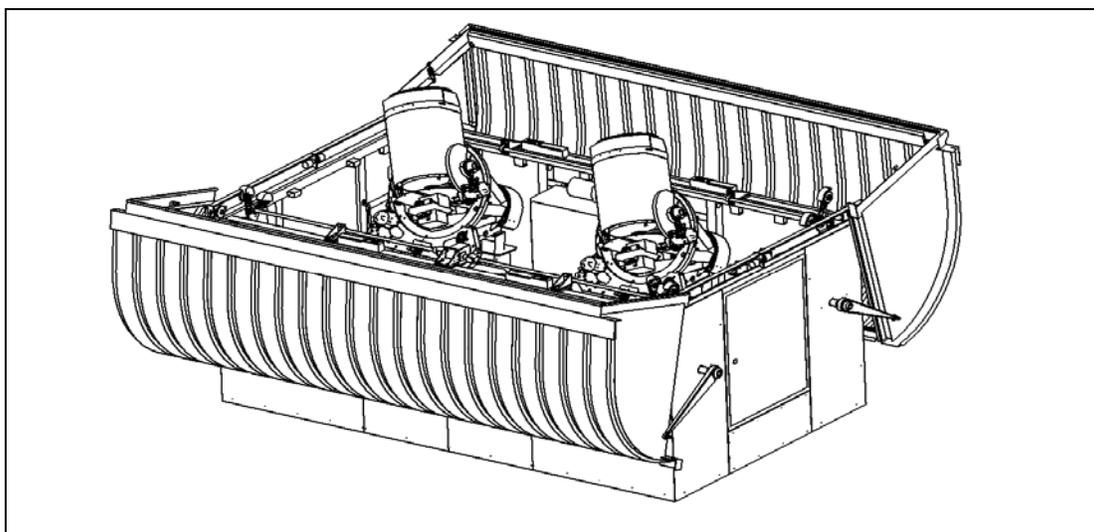
Figure 7. An isometric view of the dual 0.4m telescope enclosure called “Aqawan”, designed by Annie Hjelstrom.
