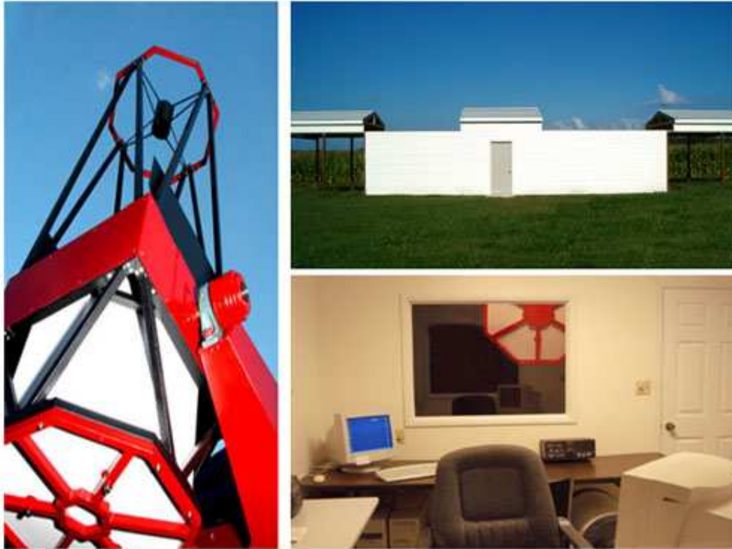
Figure 3. The 0.81-m (F/4.60) prime focus telescope at ARI (Charleston, IL) used for the IASC search campaigns.
