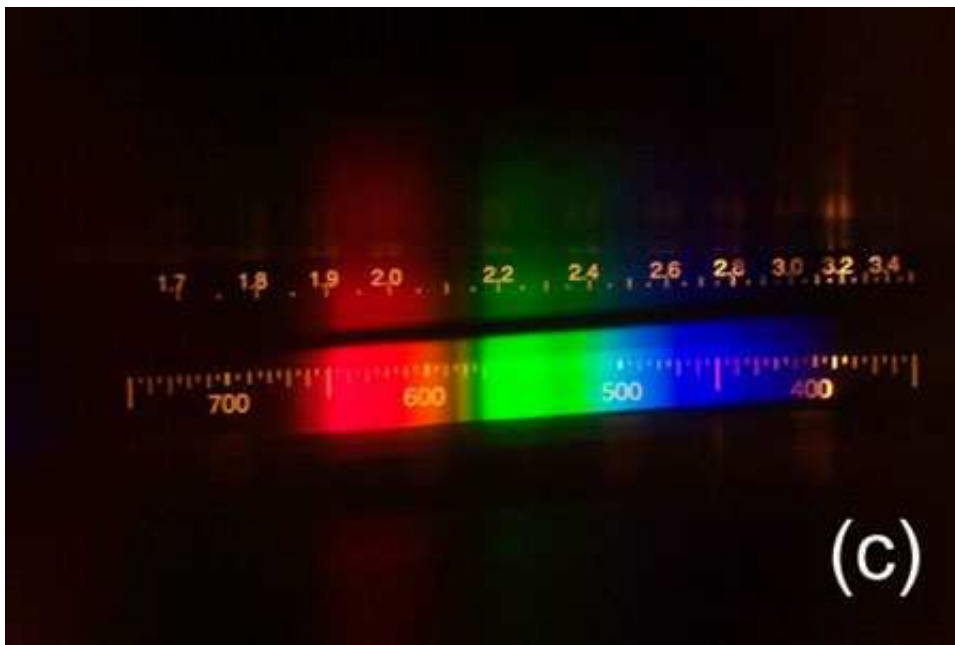
Figure 1. (a) The GE soft white and the GE Reveal bulbs. Notice the bluish tint of the Reveal bulb. (b) The spectrum of the soft white bulb. (c) The spectrum of the Reveal bulb. Notice the prominent absorption lines in the yellow.
