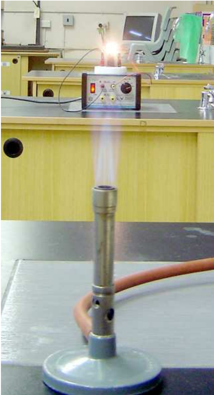
Figure 1. A light bulb appears to twinkle when observed at a distance through the turbulent air above a Bunsen burner flame.
