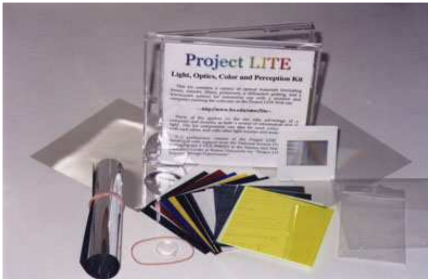
Figure 1. Project LITE Light, Optics, Color, and Perception kit. Contents include optical elements for interactive experiments with light emitted from a computer monitor.
